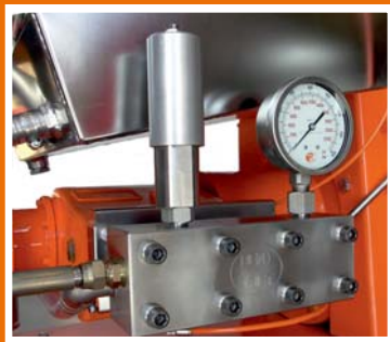
Stainless steel pump-head. Integrated cooling for plunger-seals.
